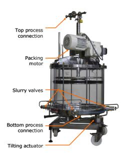
Fig.1. VERDOT Ips<sup>2</sup> InPlace column
